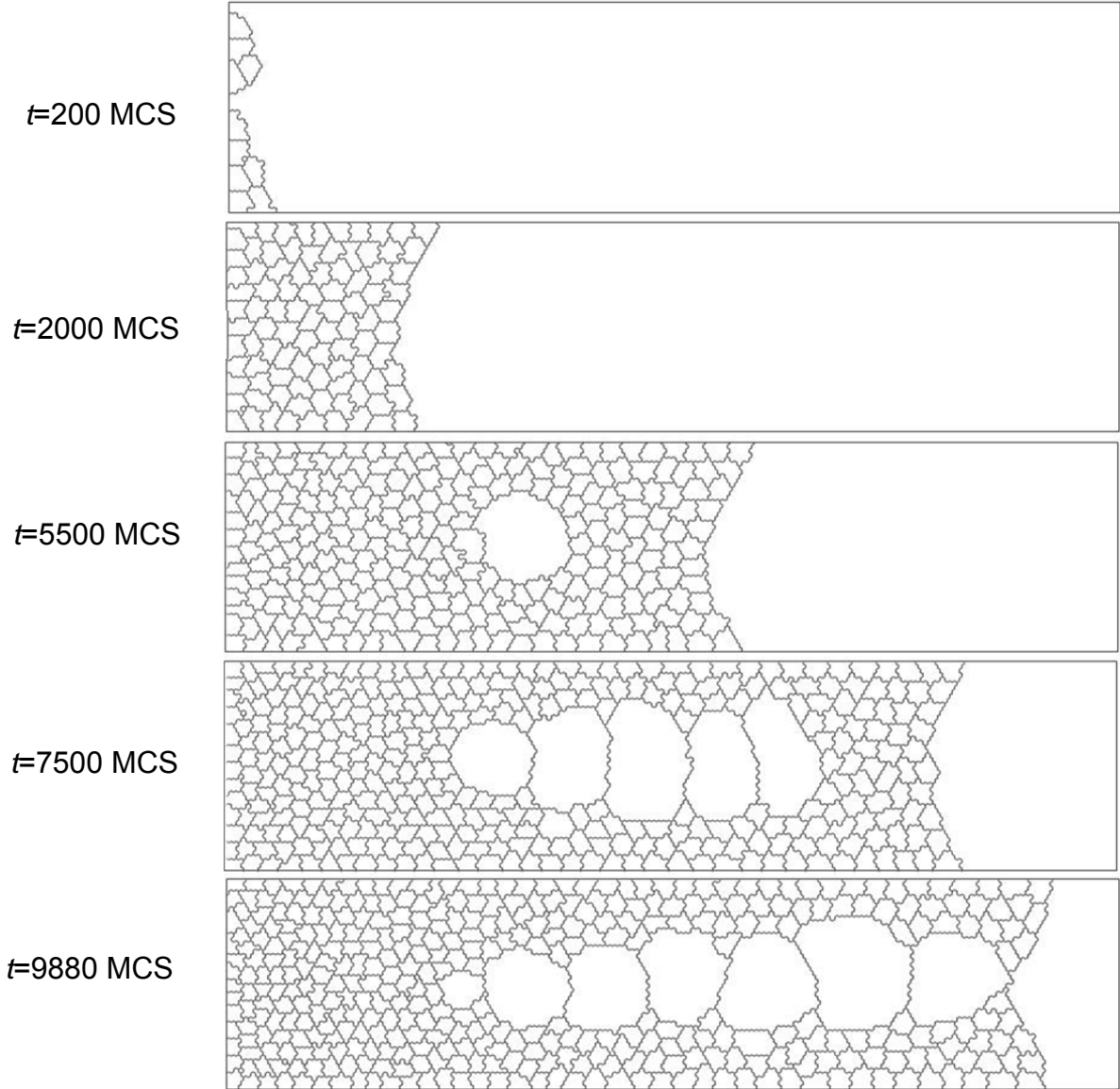
Figure 15. Results of the foam-flow simulation on a 2D 3 rd -neighbor hexagonal lattice. Simulation code is given in Listing 10, Listing 11, Listing 12, Listing 13 and Listing 14.
